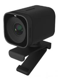
The Vidi 250 is a wide angle 4k camera designed for use with conferencing systems. Intended for huddle room or small to medium conferencing rooms, the Vidi 250 has a 120° field of view, allowing everyone in the room to be seen. The Vidi 250 uses auto framing technology to adjust the focus and zoom to keep participants in view. The Vidi 250 can be either display mounted or wall mounted.
