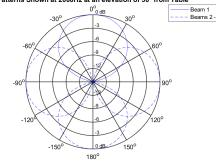
TTM-X Polar Responses at Center of Tracking Zones Patterns Shown at 4000Hz at an elevation of 30° from Table
