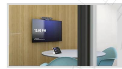
**Poly** – Presented their new MTR range of products, specifically the X70 and E70 solutions for large meeting spaces. The X70 video bar has a unique camera design with a wide angle 120 degree field of view camera and a narrower 70 degree camera to reach further into the room and these work intelligently together with Poly's Director Al technology. The E70 Camera has the same dual camera experience as the X70 but it is just the camera ready to fit with other audio solutions.
